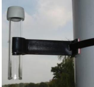
**Description:** Acrylic tube fitted with coloured and white thermoplastic rubber caps. The coloured cap contains the absorbent.
